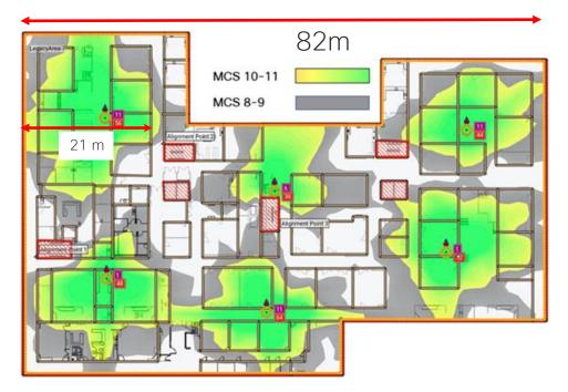
• Single-antenna devices (smart-phone) should see MCS10-11 with 40 dB SNR
