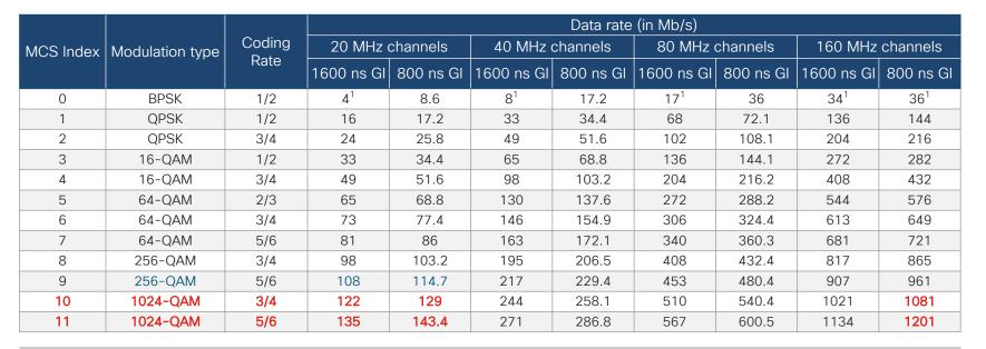
Up to 1.2Gb with 1 radio, up to 10 Gb\* with 8 radios @ 160 MHz
